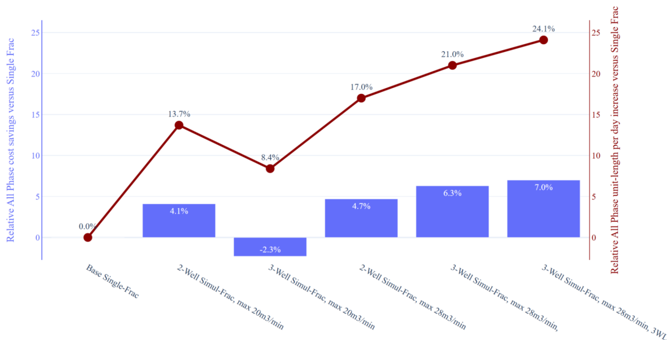
Figure 35—Scenarios' All Phase (Prep-to-Demob) cost savings and increased lateral length per day versus Base Single-Frac scenario
