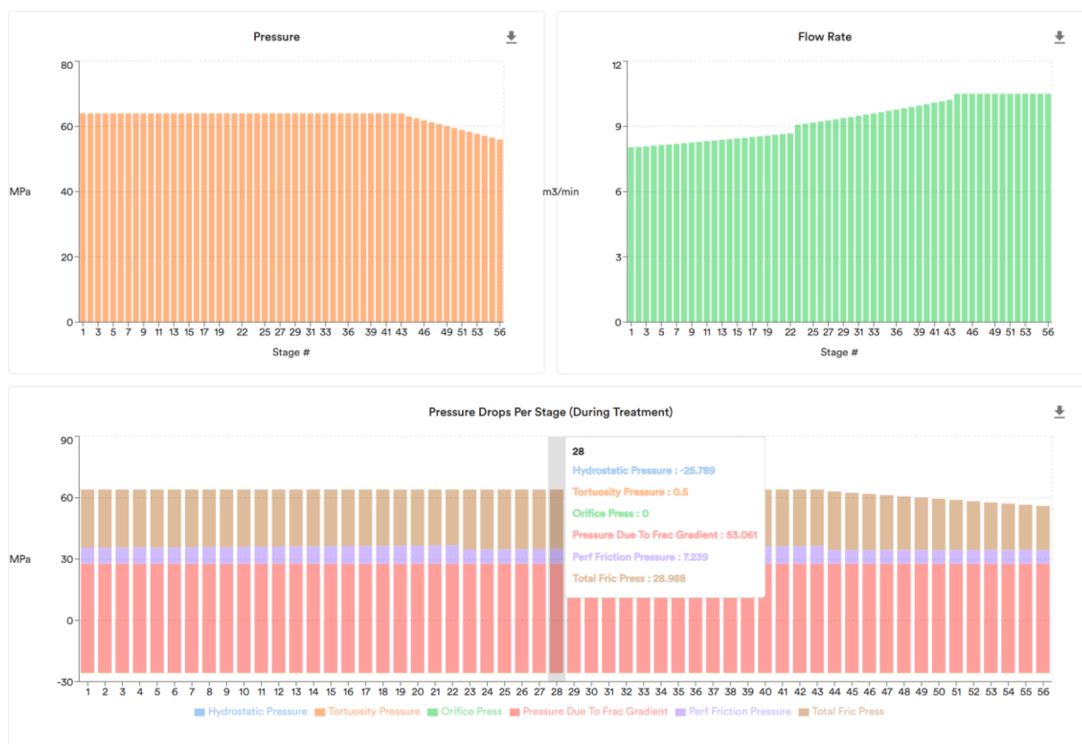
Figure 26—2-Well Simul-Frac, max 28m 3 /min scenario's treatment physics
