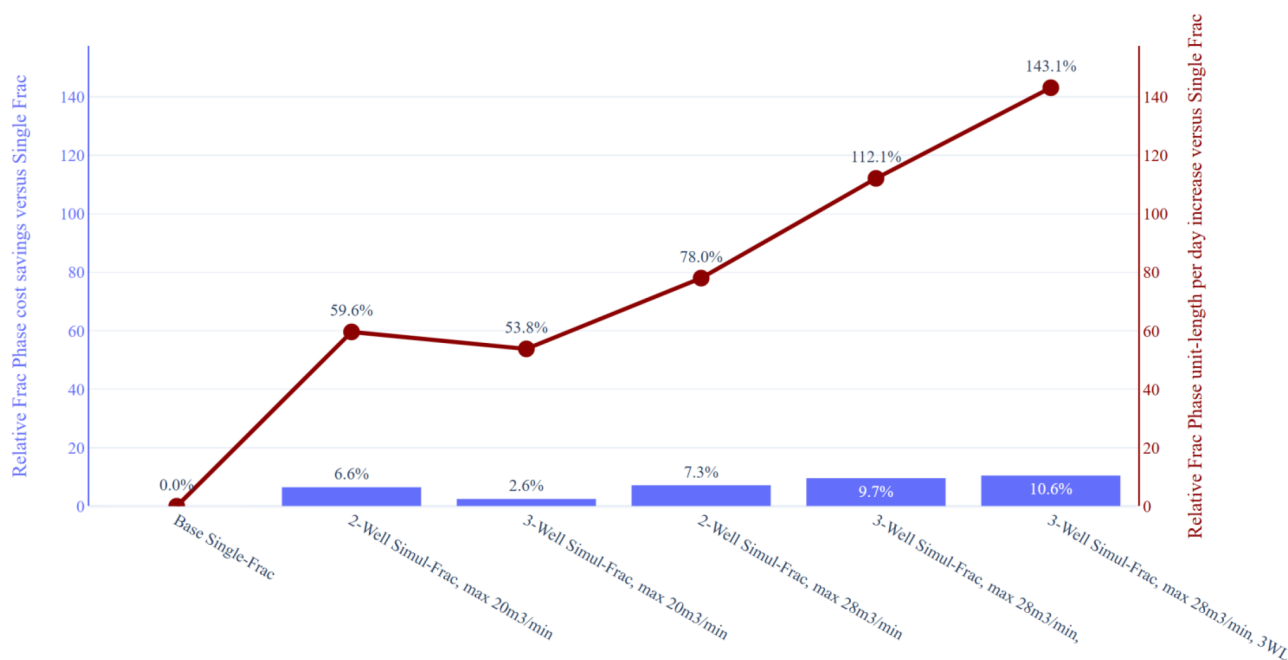
Figure 36—Scenarios' Frac Phase cost savings and increased lateral length per day versus Base Single-Frac scenario
