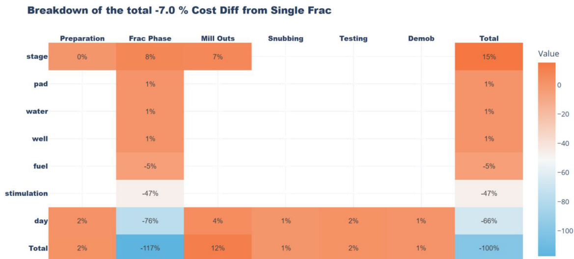
Figure 34—Breakdown of cost difference between 3-Well Simul-Frac, 28m 3 /min, 3WL and Base Single Frac scenarios
