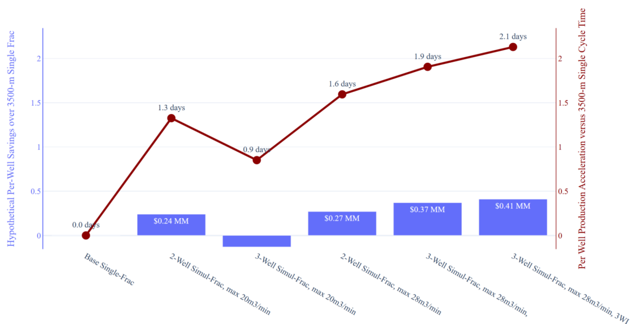
Figure 37—Absolute all-phase, per-well completions cost and cycle time savings over hypothetical 3500-m single-frac completion
